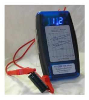
Very similar accurate circuit and features of the EVB meter. User-Unfriendly ESR chart. Alligator clips are not suitable for in-circuit testing. Bulky. Heavy, and Much too expensive, when compared to the EVB meter. Bonus – build-it-yourself kits are available!
