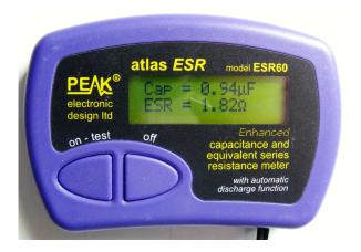
Compact. Accurate. Measures Capacitance up to 22000uf (but not in-circuit). High-quality parts, but impossible to repair by the owner. 12V battery life is not great. Measures up to only 20 ohms ESR. Does not measure capacitors with less than 1uf capacitance.
