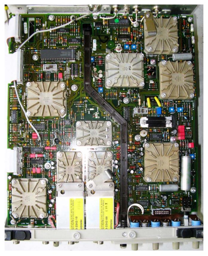
Here is the A1 Main PCB after restoration. The new heat-sink is evident to the right of the kink in the black plastic stem for the On-Off switch. All the new electrolytic capacitors are also clearly visible.
