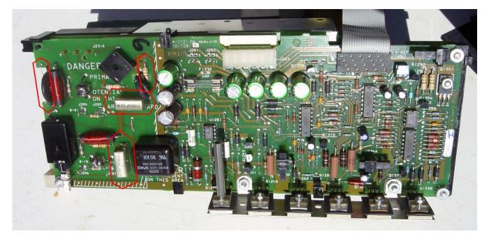
Here is the A2 PCB before restoration, with the AC High-voltage section on the left.
