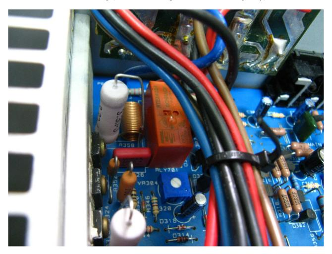
Here, also clearly visible at the Power Amp circuits, are the upgraded 3.3 ohm Metal-oxide power resistors, the orange Vishay CPF Metal-film low-noise power resistors, the Blue Bourns Cermet trimmer, and the tan Vishay CMF Metal-film resistors, which replaced ALL the original noisy carbon resistors in the audio-signal path.
