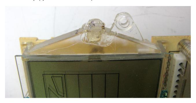
At an easy low-stress current of only 14.5mA, the LED's are very bright, even for daylight, and enhance the contrast and readability substantially.
