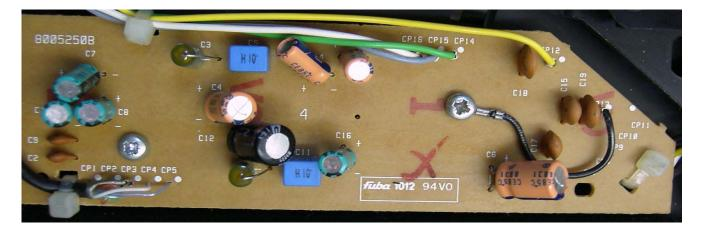
Basically, I replaced all the Electrolytics with Nichicon HE, and Wima MKS2 (red); the ceramics with Panasonic ECQP (brown) film caps. C2 and C9 got special treatment and were replaced with Mica caps, as they have to be very stable in the oscillating circuit.
